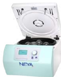
Centrifuga ventilada NEYA 8 BASIC, 4x175 ml, 6000rpm
